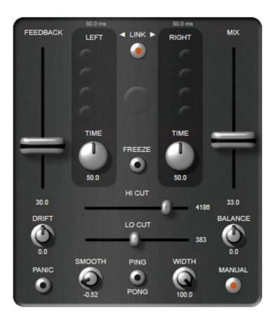
In manual mode the delay time selection controls are replaced with one single dial "**TIME**" for each channel.
